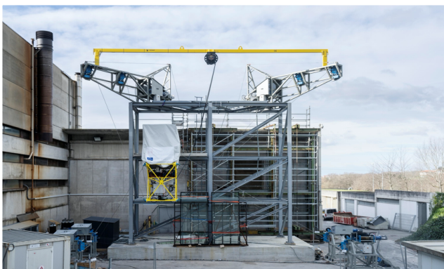
Figure 1: Hephaestus cable robot overall system with an example of a prototype building and curtain wall system, suitable for robot assembly
