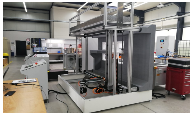
Figure 2: A 1:2 semi functional prototype of multifunctional façade processing robot was built and tested in laboratory as a proof of concept
